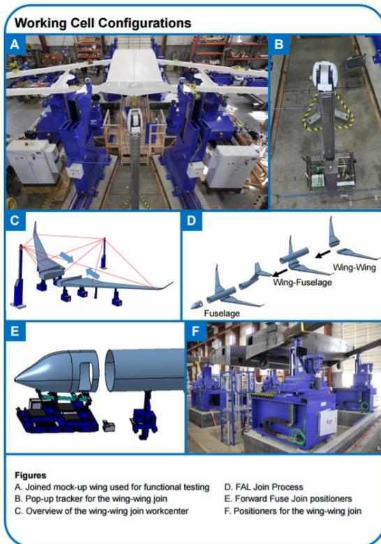
**Figure 1 Image Courtesy of Electroimpact**
